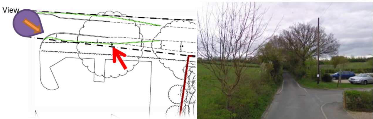
Figure 2. Road widening is not practical without severe impact on the surrounding land, possibly requiring additional earthworks to areas beyond the ownership of Highways and the destruction of mature trees.
